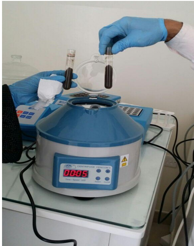
Fig 3: Centrifugal method to separate solids and water.
