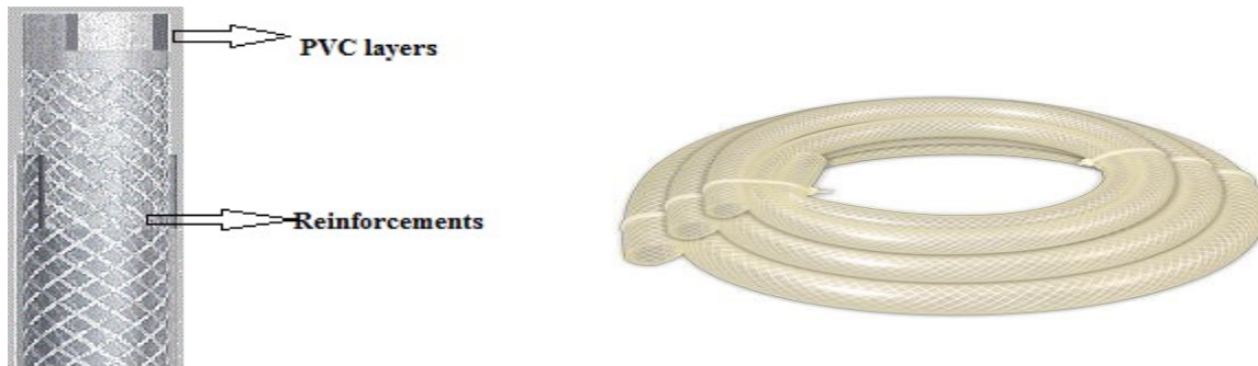
Fig. 17 –Braided hose pipe Structure
