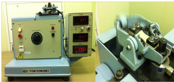
Figure 1. Plane bending fatigue testing machine
