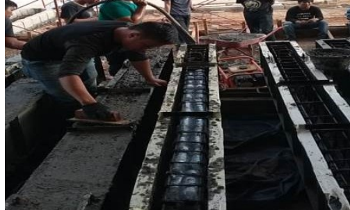
Figure 5. Casting of specimen.
