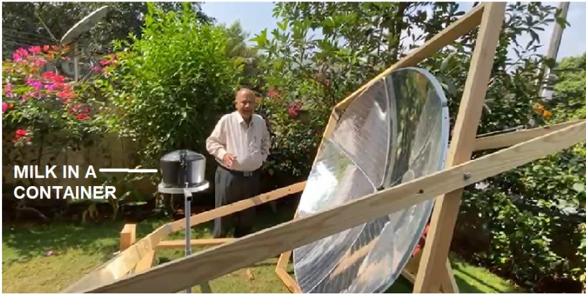
FIG 13 HEATING OF MILK IN THE PRESSURE COOKER BY THE REFLECTED RAYS FROM THE PARABOLOID
