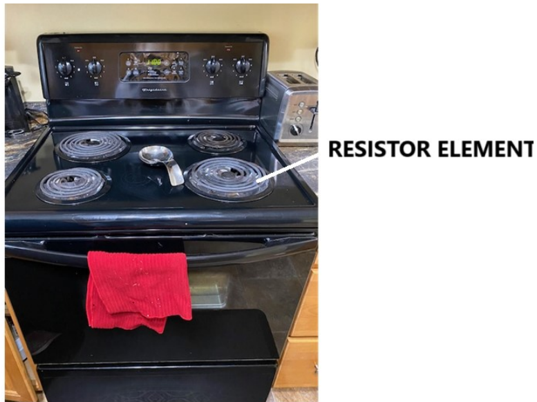
FIG 9 COOKING STOVE WITH RESISTOR HEATING ELEMENT
